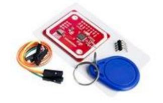
PN532 NFC RFID module V3, NFC with Android phone extension of RFID provide Schematic and library
